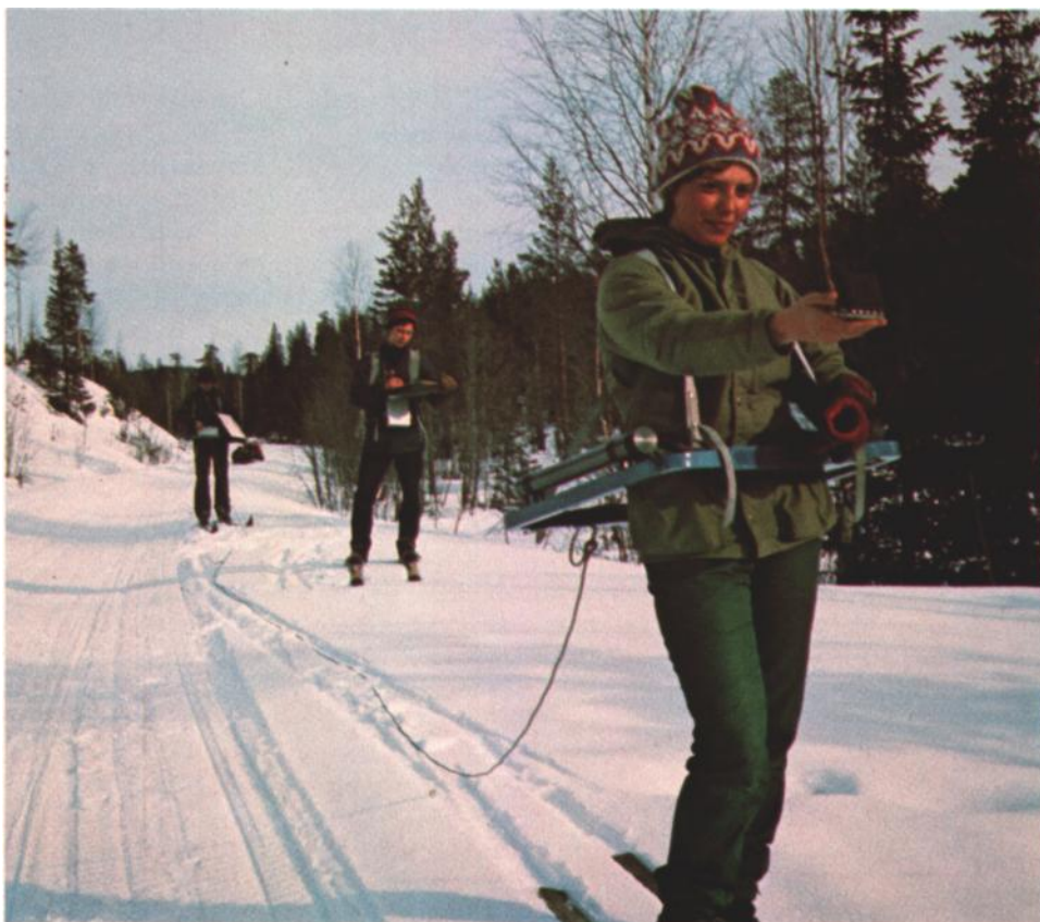
FIG. 2. Special geophysical methods are called for when conventional methods fail. A. A pulse electromagnetic receiver in use in a Finnish forest. B. An electromagnetic ("Slingram") measuring crew at work in northern Sweden. Photo: A. Hesselbom)
