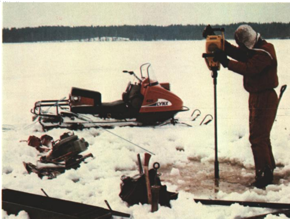
FIG. 3. Geochemical exploration goes on all year. Sampling lake sediments through winter ice in a Finnish lake.
